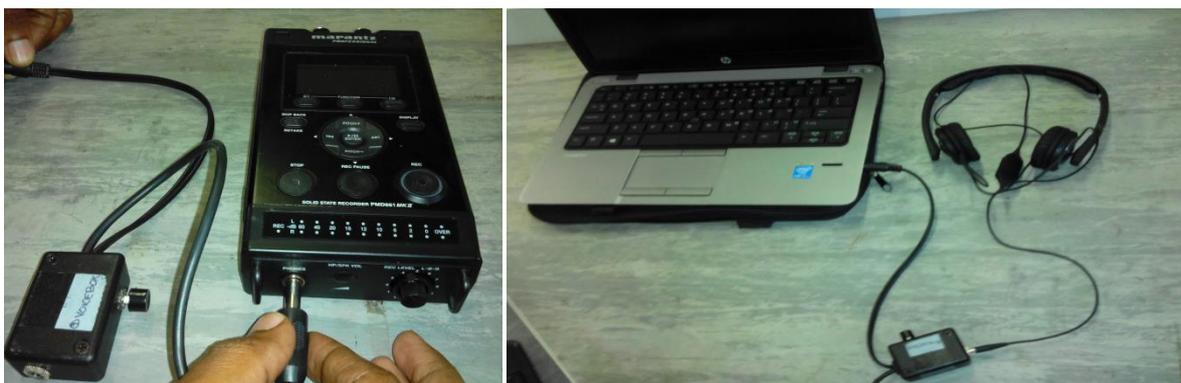
Connect the **large plug** to the Marantz whilst the **smaller plug** is connected in to the **Laptop audio port**. The **headset** is then connected to the **voice box**.
